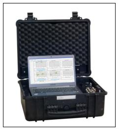
system "PD-Expert" used for automatic diagnosis of insulation defects in high-voltage equipment. This intellectual expert system is very important for the staff with little experience.
