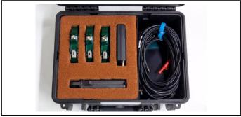
The "PD Sensors - CL" sensor set is used for measurements in the high-voltage cable insulation. It includes three "RFCT-4" sensors, a leakage capacitive current sensor and a "GTI-R" calibrating generator for long cables' calibration.
