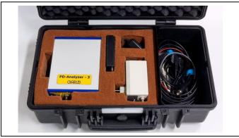
The "PD-Analyzer-3" device is supplied in the protective transportation case.
