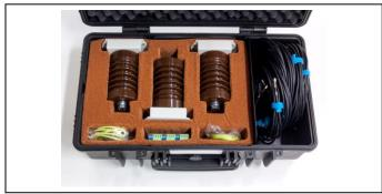
The «PD Sensors - RM» sensor set is used for measurements in stator winding of high-voltage electrical machines. It includes three "CC-12/U" highvoltage coupling capacitors and one "DRTD-3" sensor. "DRTD-3" is used for connecting to the temperature sensors build into the stator winding. In this case the temperature sensors operate as the antennas for PD measurements inside the winding.
