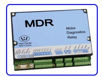
The complete version of the «MDR» device for the stator winding insulation monitoring is a finished module with the dimensions of 250 \* 200 \* 45 mm. The connection of all the sensors and links is done with the standard screw terminals.
