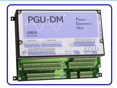
The insulation condition monitoring «PGU-DM» system is a device installed into the enclosure.
