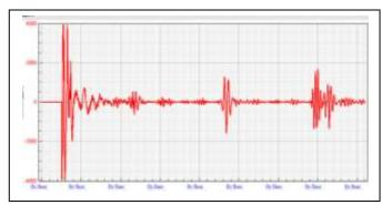
For better noise rejection, several pulses are sequentially injected into the line, which allows them to be averaged by statistical methods.
