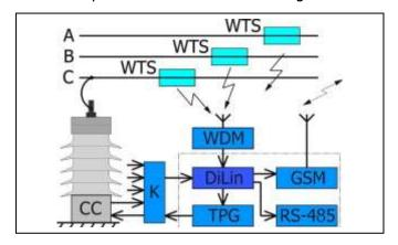
Coupling Capacitors (CC) are used as the primary sensors in the DiLin system. The number of coupling capacitors used corresponds to the number of power line wires monitored.
