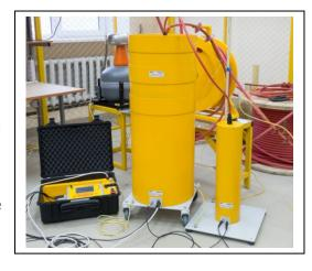
As a result, resonance arises in the circuit, which consists of the monitored cable capacity and coil inductivity. The monitored cable is influenced by sinusoid damping AC voltage (DAC) with the oscillation frequency from 50 Hz to 1000 Hz, in dependence of the tested object capacity (i.e. the cable length).
