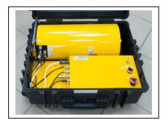
Measuring process is controlled from the PC laptop by WI-FI for safety. PD signals are saved and analyzed on the PC laptop. The data can be viewed and processed in the field during the measurements or later in the office.
