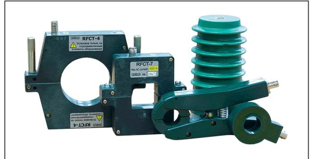
«RFCT-7» is split-core sensor with a 34\*34 mm inner window. The sensors measure partial discharges in conductors which have power current up to 1000 A. They are specially designed for cable insulation monitoring systems.
