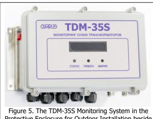
Protective Enclosure for Outdoor Installation beside the Transformer. - Transformer load monitoring by the IFCT-5 sensor (Figure 4).
