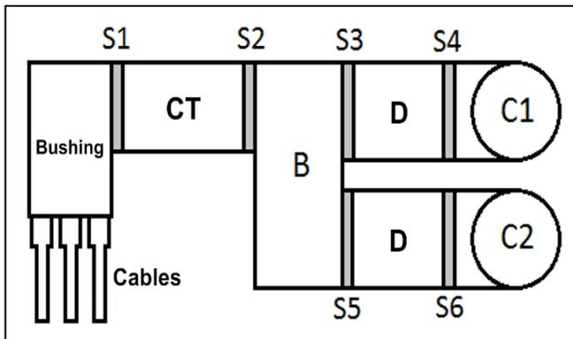
The monitored gas-insulated section consists of cable terminations, a measuring current transformer (CT), a breaker (B), and two breakers (D) for the commutation of the bus sections (C1-C2). The six sensors (S1-S6) provide the GIS insulation condition monitoring, defect location, as well as HV cable insulation condition monitoring.
