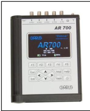
“AR700” device is used for measuring of acoustic signals on the external surfaces of gas-insulated breakers and substations, power transformers and other tank high-voltage equipment. The acoustic signals are caused by partial discharges in the insulation, which is the sign
